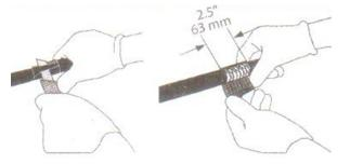
Install the grounding strap to the outer conductor of cable. And then use cable ties to fix tightly.
